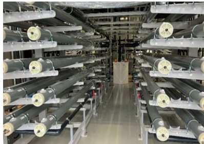
Concentration of liquid fertilizer using UF membrane system
