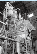
Large-scale falling-film vacuum distillation equipment
